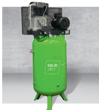
SOLIDbase 680-10 ST/870-10 ST / 530-15 ST/680-15 ST 4 space saving stationary piston compressors with vertically mounted receivers, 10 and 15 bar, including star-delta protective combination (5.5 kW version completely prewired with compressor), Condor quality pressure switch including operating hours counter
