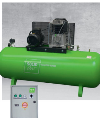
SOLIDbase 520-10 to 1300-10 / 460-15 to 1000-15 12 stationary piston compressors with horizontally mounted receiver, 10 and 15 bar, incl. star-delta protective combination (5.5 and 7.5 kW completely prewired with compressor) Condor quality pressure switch including operating hours counter
